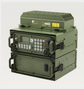
The 2110M-B125 is a compact 125 watt base station syster utilising the 2110M manpack radio and the 3160 125 watt power amplifi er. Coupled with Codan's 3520 power supply, the system is operational from DC and AC mains supplies, auto switching to DC with loss of AC.
