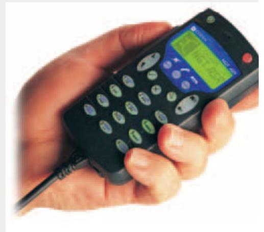
The atmospheric noise to which all HF radios are susceptible can make communication over an HF radio difficult. The result of this atmospheric noise is difficulty in understanding the other party. CODAN has developed 'Easitalk', which reduces the noise on the HF medium. Easitalk processes the received audio signal. Easitalk is a standard in-built feature that can be turned on or off at the press of a button. No other user action is required.
