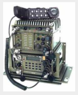
This mobile package with maximal output power of 25 W can be installed in all wheeled and tracked vehicles. The AT RF13 transceiver and ATZM13.1 amplifier are located on top of each other in a springcushion frame. If the mobile set is designed for installation in wheel vehicles without artillery or mortar weaponry, c for fixed posts, you may use the lighter, non-cushioned frame 7007.100.01 instead of springcushion frame 7007.100.10. The set can be controlled from one location.
