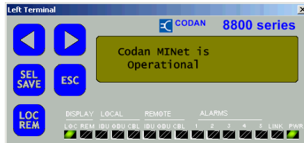
Figure 7: LCD and keys on the IDU
