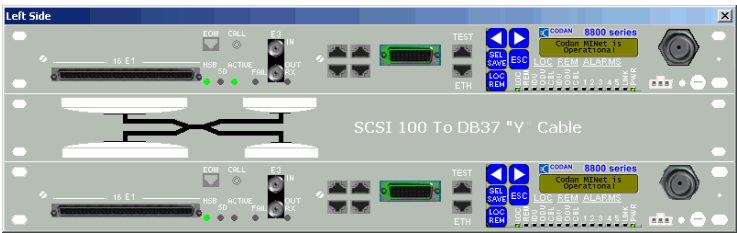
Figure 6: Front panel of the IDU in a 1+1 system
