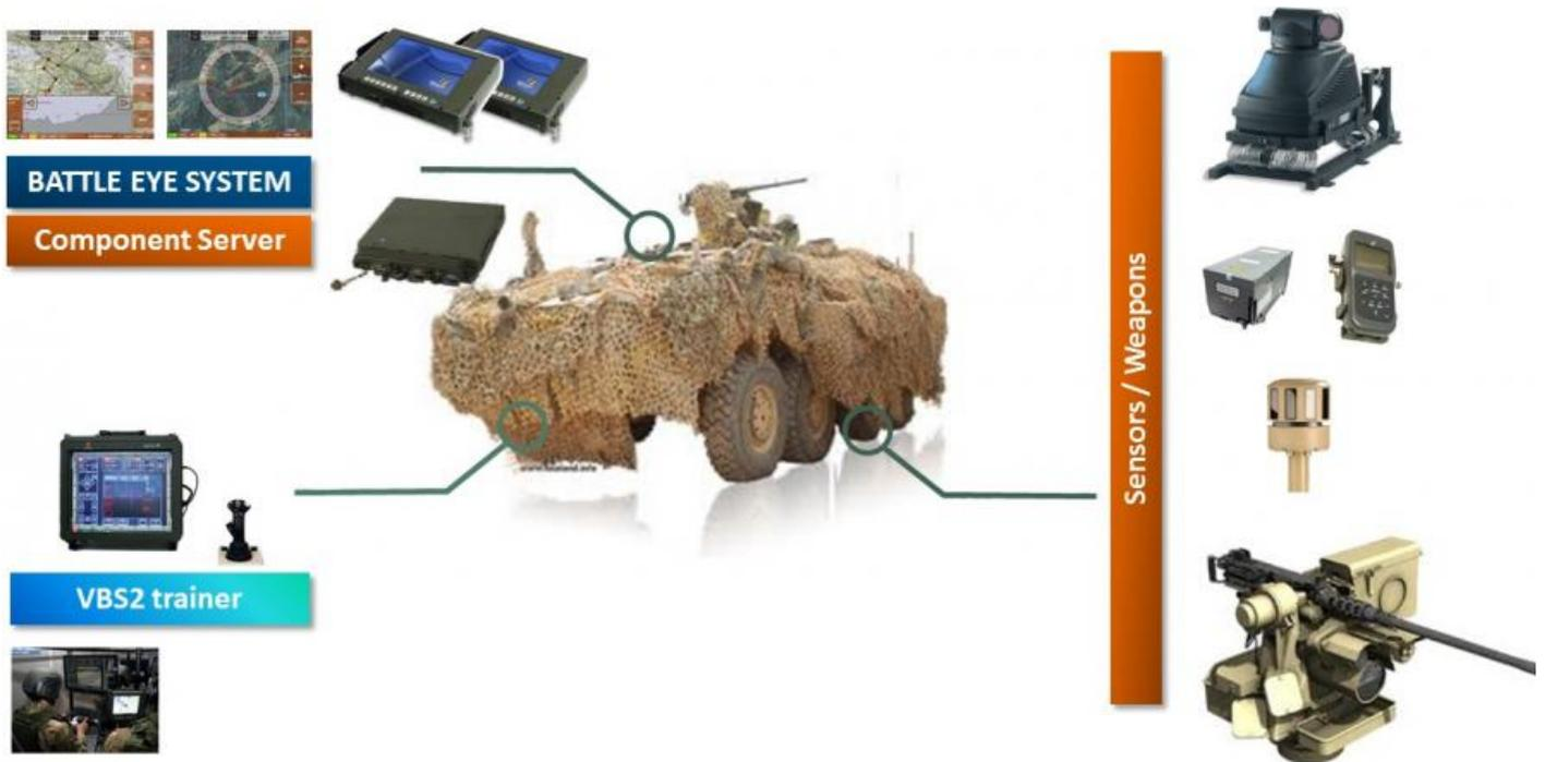
Every sensor, device or weapon system is connected to a Component server via specific device driver. Component server then exposes common API towards Battlefield Management system.
