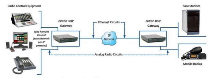
AT Radio dispatch console or desktop remote (up to two positions) extended over IP.
