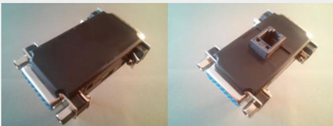
The AT Voice USB-Logger is a simple device designed to provide time stamped recording and metatag logging of voice and data communication. The AT USB-Logger includes a simple software program installed on a PC that connects through the AT Voice USB-Logger to your communication transceiver eg Codan Envoy or NGT.
