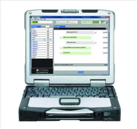
Codan's SprintChat and SprintNet applications utilise the benefits of the 3G ALE waveform to provide fast, secure and a highly flexible approach to HF data communications. Peer-to-peer email, file transfer and chat data formats are supported as well as phone SMS and internet mail via the SprintNet gateway. The flexibility and interoperability benefits of the Sprint solution provides a powerful extension to your HF network capabilities.
