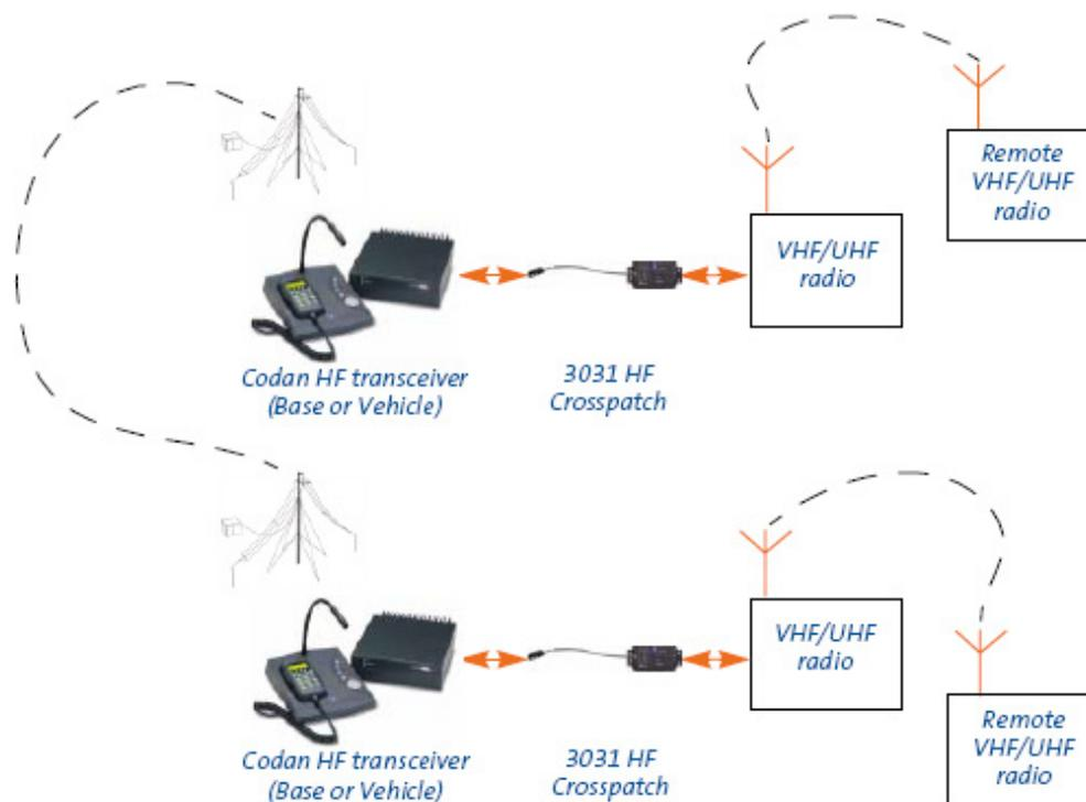
NOTE: The HF transceiver must be a Codan NGT/2110 model that has a General Purpose Input/Output (GPIO) port, such as the NGT SRx, SR, ASR and 2110 series Transceivers.
