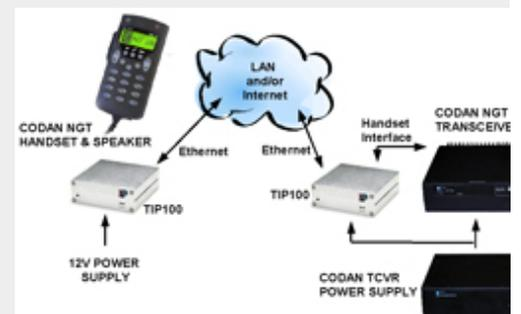
Information that the transceiver sends to the LCD display of the handset is relayed via the network and displayed on the remote handset. Similarly, button presses on the remote handset are relayed to the transceiver as if it was a locally attached handset.
