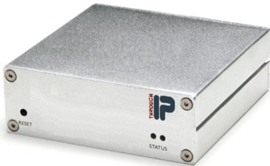
Set up consists of plugging the AT IP1 in to the Ethernet network and connecting it to the transceiver handset and speaker connector through the supplied cables and plugging it into a 12V DC power supply. Then it is only a few easy steps to find or set-up the IP address for the unit. From there further configuration is through a web browser attached to the network.
