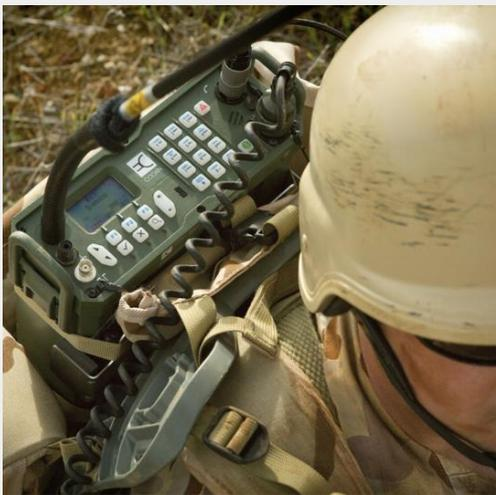
The waveform is based on the Standard NATO Agreement (STANAG 4538) and is available as an option for the Codan's 2110M series HF man pack radio. The (3G) automatic link establishment (ALE) supports enhanced data throughput and linking performance over noisy HF Skywave channels. Integration of the ALE linking protocol and the data transport mechanism provides effective increased data throughput and shorter linking times in difficult HF conditions.
