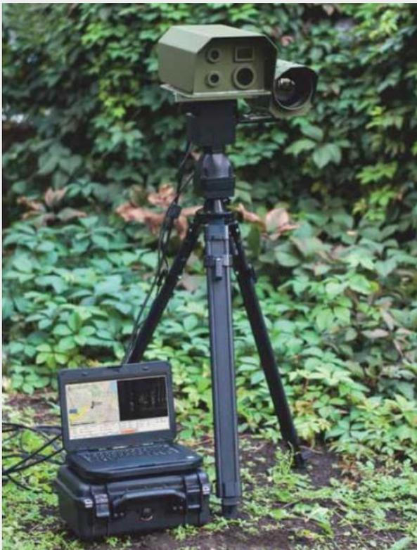
The complex is a multifunctional optoelectronic device designed for twentyfourseven video monitoring of the terrain aims searching and automatic detection of camouflaged optical aiming and tracking devices, determination of their coordinates and distance in difficult terrain and urban buildings conditions.
