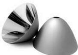
The outstanding reflector performance has been accomplished by using electroforming technology and high reflectance in the visible spectrum through a special Al coating and protection layer. The reflector surface is without visible distortions, resulting in exceptional beam geometry and efficiency.
