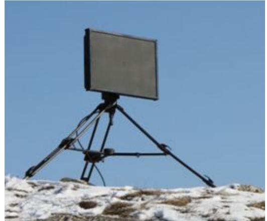
**AT MGSS Mobile Ground Surveillance System - Intercepting Detecting Radar**
