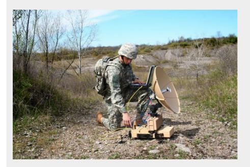
Providing high-speed data communications in a portable package, the Panther™ .96 VSAT terminal is perfect for military missions or business requirements. Extremely rugged and lightweight, the Panther™ VSAT terminal offers Internet and VPN connectivity, enabling video transmission with Inmarsat BGAN-like simplicity, but with significantly higher data rates over commercial and military satellites.
