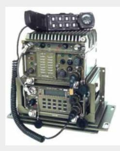
This mobile package with maximal output power of 50 W can be installed in all wheeled and tracked vehicles. The AT RF13 transceiver and AT ZV13.1 amplifier are located on top of each other in a spring cushion frame. If the mobile package is designed for installation in wheel vehicles without artillery or mortar weaponry, or for fixed posts, you may use the lighter, non-cushioned frame 7007.100.01 instead of spring cushion frame 7007.100.10. The package can be controlled from one location.
