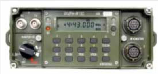
AT RF13D is a VHF transceiver designed for duplex data operation. AT RF13D design is based on AT RF13 transceiver, the difference being in an added independent input for receiving antenna, modified AF paths and modified control program. It is used in a set with ZM13.1 (ZV13.1) power amplifier, AF13, AF13.1 co-site filters. The transceiver can be operated independently with RF13 transceiver accessories.
