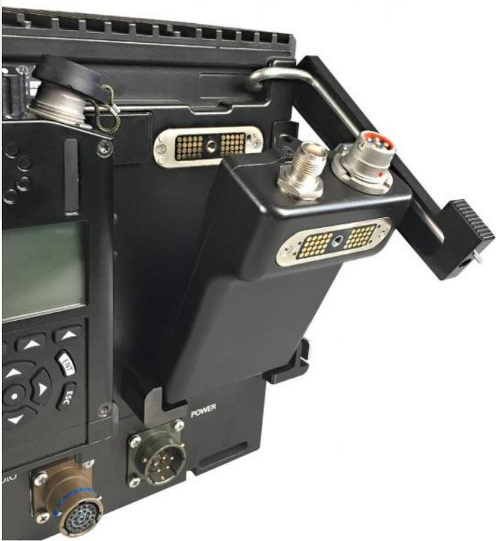
Expands the radio features according to actual mission needs. Open platform for installation of custom specific devices of different types. MM40W Mission Module type offers second independent broadband radio channel for voice and data transmission in MANET-type network. Available in L-band or S-band frequency configuration allowing data transmissions in dozens of megabits depending on the radio channel bandwidth setup.
